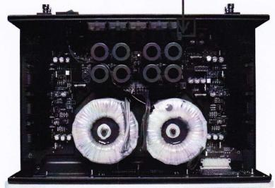
3- PLACE THE PHONO STAGE ON THE ORANGE CONNECTORS OF THE MAIN BOARD. (ONLY ONE WAY POSSIBLE)
